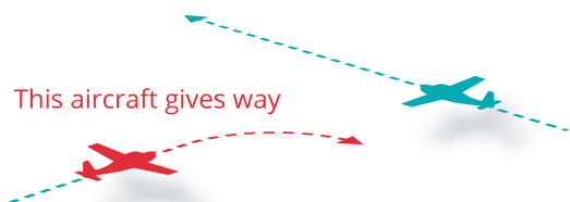
Figure 6: Aircraft with right-of-way to maintain heading and speed
