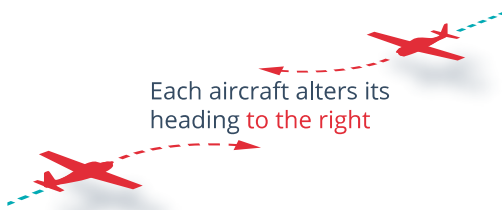
Figure 8: Aircraft approaching head-on to alter heading to the right
